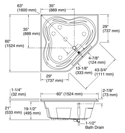
No change in measurements if connected with drain illustrated. (K-11677)
